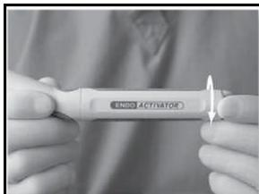
To remove the battery housing, firmly grasp the contra-angled portion of the handpiece with one hand and begin turning the non-removable, screw knob counterclockwise with your other hand.
